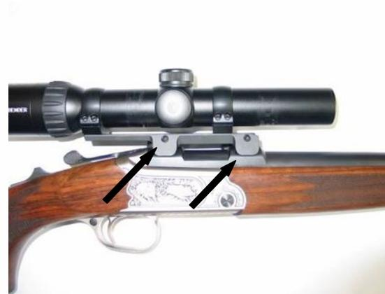
If the torque of the two levers requires adjustment, the 3-mm internal hexagonal bolts on the right-hand side must be removed. Turning the two bolts behind will adjust the torque.
