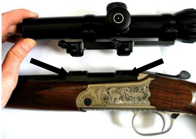
The scope mounts are attached by inserting the two lugs into the corresponding grooves.
